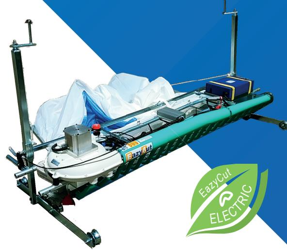
The EazyBattery system operates at two speeds. The electric motor can also be powered by a 230V connection. In this setup, a fixed-frame EazyFrame can be considered so that cultivation tables or conveyor belts can move underneath.
